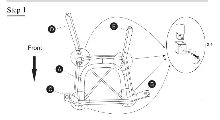
Turn Seat (A) upside down onto a clean, non-marring surface. Place Front Legs (B/C) and Back Legs (D/E) in corresponding positions on bottom of Seat (A).
